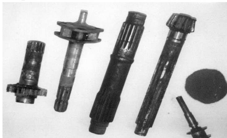
Fig. 3. Sample with welded powder material
