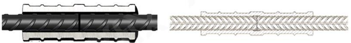
Connecting reinforcement for concrete with crimp couplings
