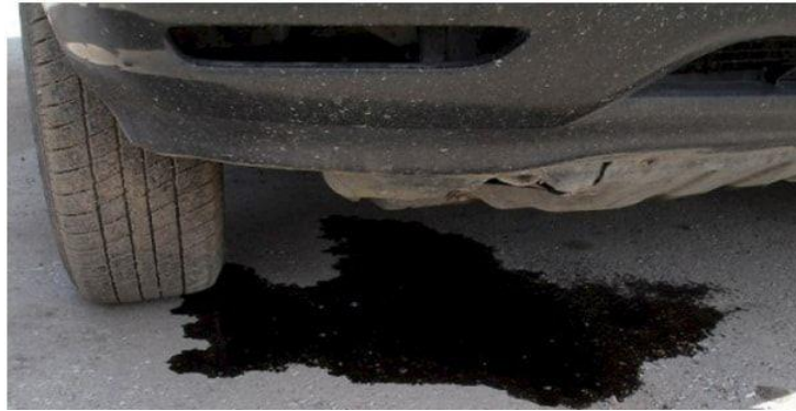
Picture 1. Oil leakage due to loss of oil filter tightness
