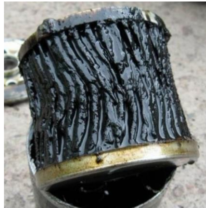
Figure 3. Contamination of the oil filter with thickened oil
