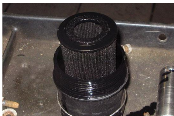
Figure 2. Oil filter contamination with wear products
