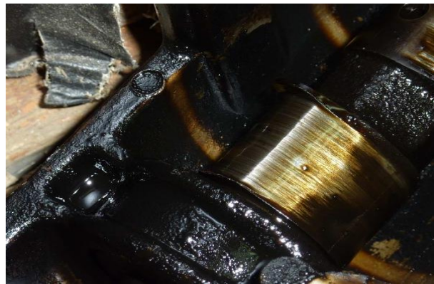
Figure 5. camshaft cam due to lack of oil supply
