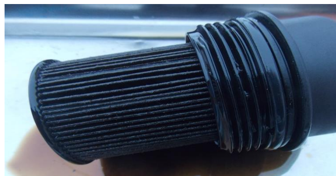
Figure 6. Oil filter element in normal condition after exhaustion of its life
