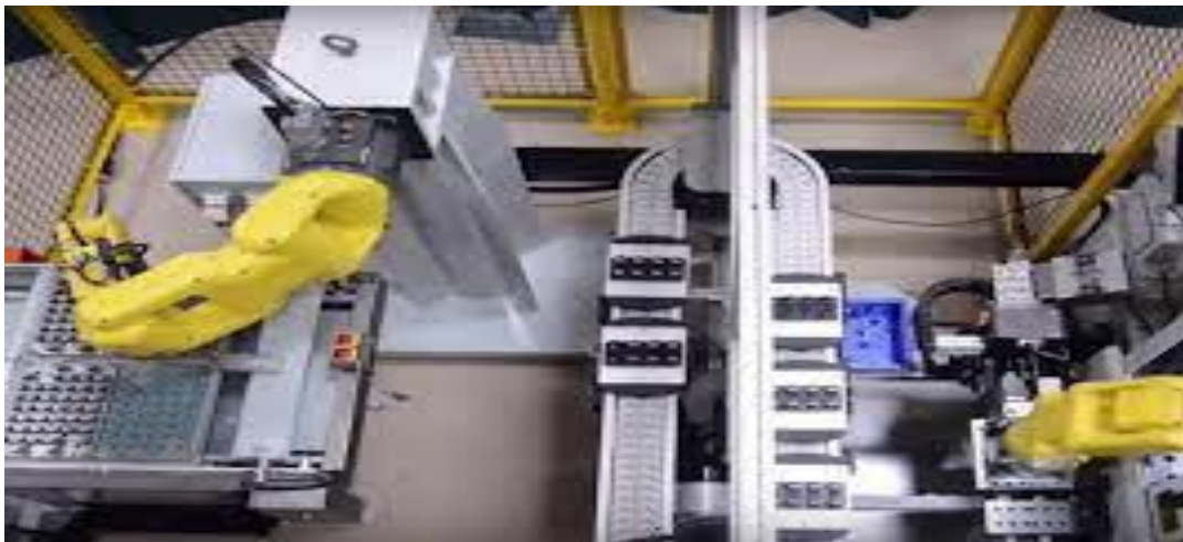
Figure 1—Robot manipulator sets the workpiece into the machine The principle of operation of the robot-manipulator and its control.
