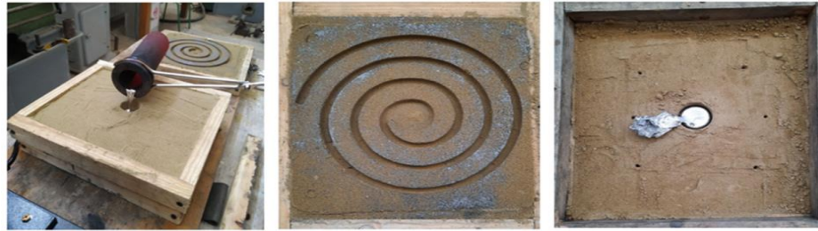
Figure 2. The process of pouring sand-clay mixture into the sample. a - casting process; b - spiral sample; s - cast sample.
