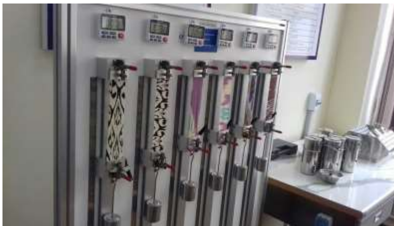
Figure 9. The process of checking the elongation of the fabric at break.
