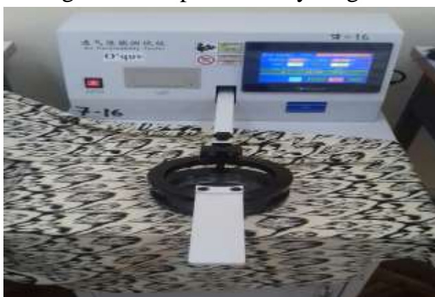
Figure 8. The process of testing air permeability
