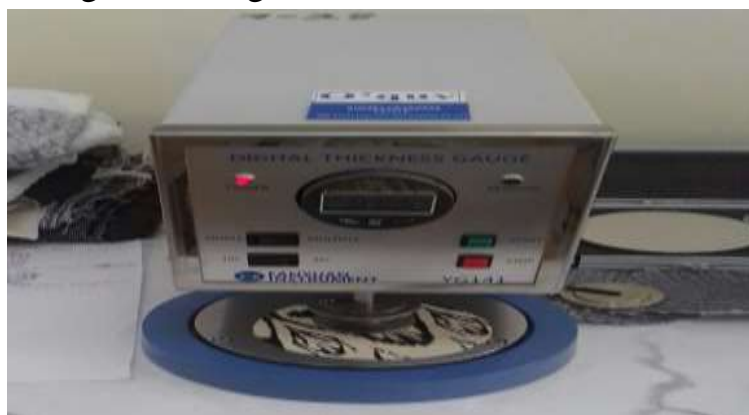
Figure 3 The process of checking the thickness of the fabric.
