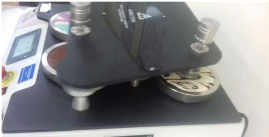
Figure 6. The process of checking the abrasion resistance of samples.
