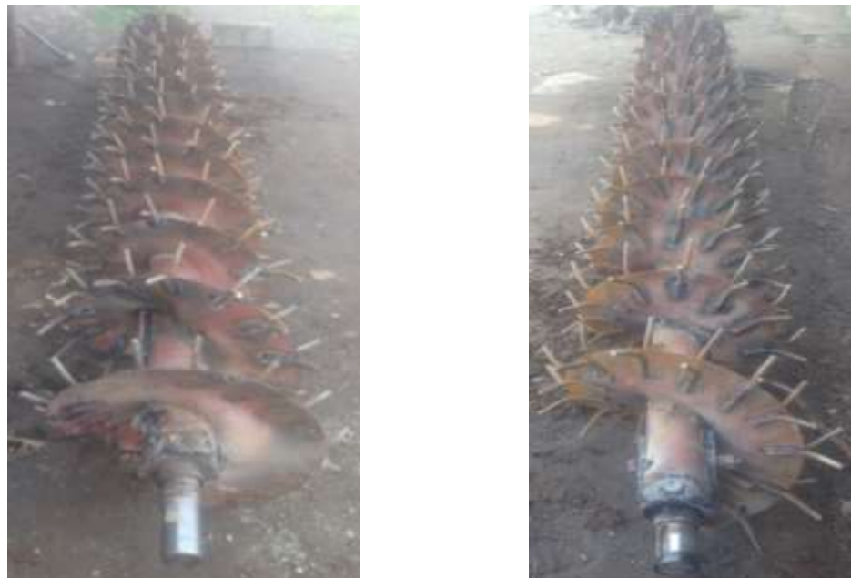
Figure 2. Prepared fresh pile auger
