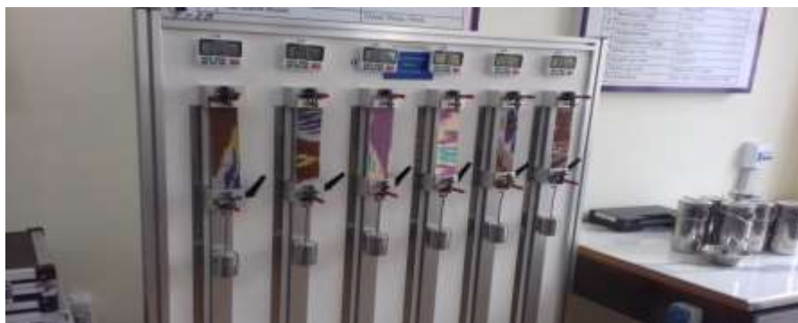
Figure 9. The process of checking the elongation at break of the fabric.
