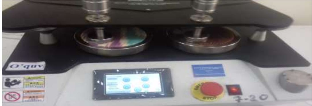
Figure 6. The process of checking the abrasion resistance of samples.
