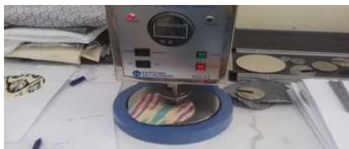
Figure 3 Fabric thickness measurement device
