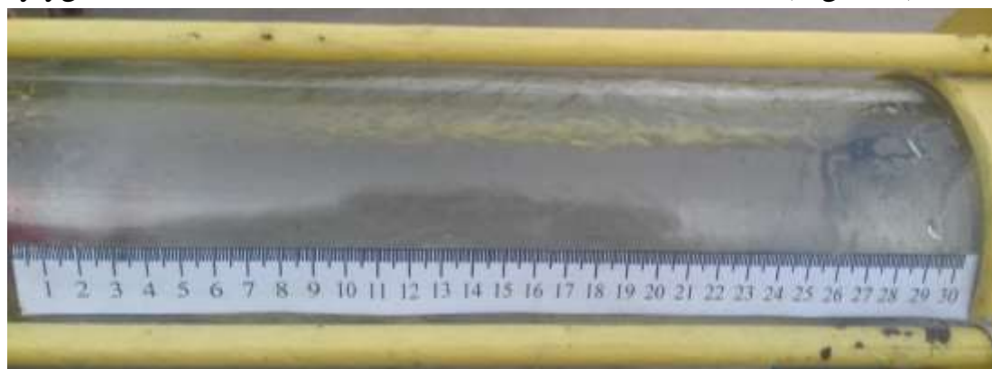
Figure 1. View of the length of the liquid film formed in the working chamber of the apparatus.
