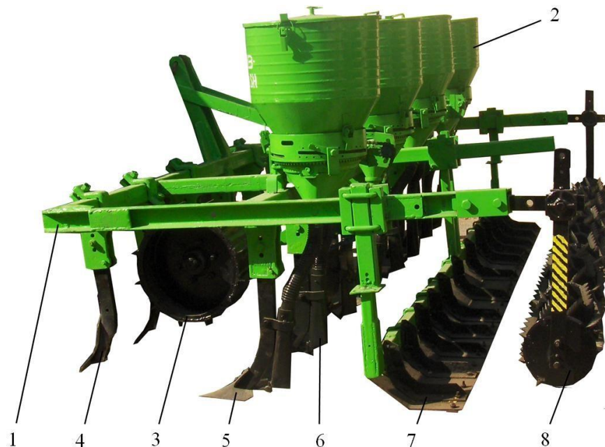
1-rama; 2- fertilizer spreader; 3- base wheel; 4-5- soil softening working bodies; 6- soshnik; 7- leveler; 8-toothed-plank reel.
